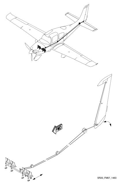
Figure 7-3 Rudder Control System
