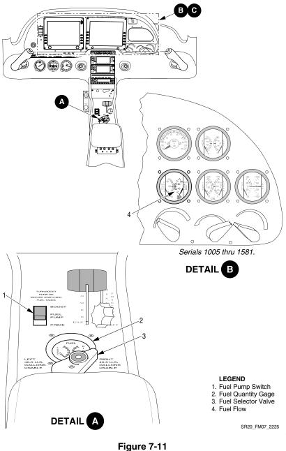
Figure 7-11 Fuel System Controls and Indicating (Sheet 1 of 2) P/N 11934-003 Revision A5
