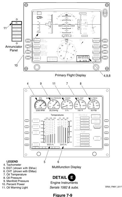
Engine Controls and Indicating (Sheet 2 of 2) P/N 11934-003 Revision A5
