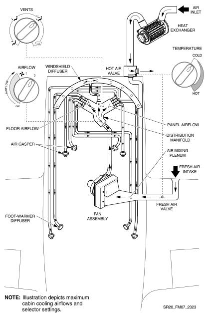
Figure 7-14 Environmental System - *Serials 1639 thru 1885* P/N 11934-003 Revision A10
