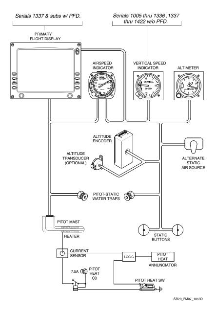
Figure 7-16 Pitot-Static System Schematic
